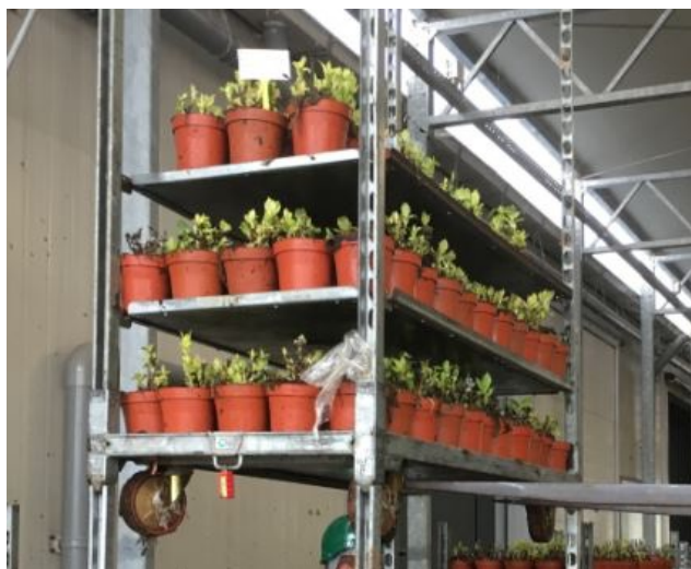
Whole DC / CC container stacked without connecting rod.
