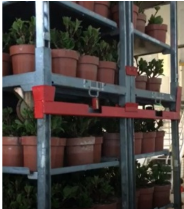
Foto: Stacked whole DC / CC containers with connecting rod.
